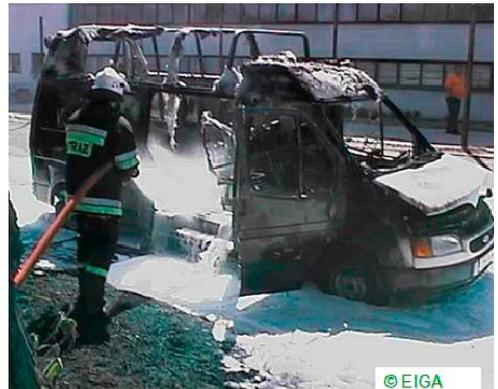
Acetylene gas leaking from the valve of a gas cylinder ignited inside a delivery van. The driver narrowly escaped. The vehicle burned out in just two minutes.
